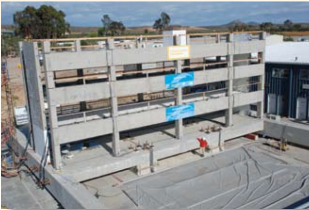
A one-half-scale parking structure underwent seismic testing on the shake table on May 7, 2008, at the University of California at San Diego's Englekirk Structural Engineering Research Center.
